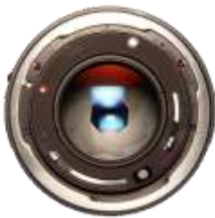
Iris diaphragm inside the camera lens
