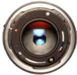
Iris diaphragm inside the camera lens
